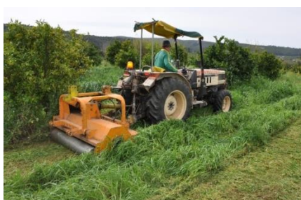
Picture 2. Mowing of vegetation covers with tractor-adapted mowers. Photo: Vercher, R., Ecovalia
